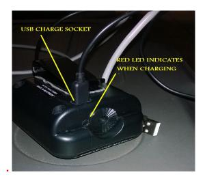
YOU CAN ALSO USE NON-RECHARGEABLE TYPES IN THIS UNIT EG THE ALKALINE 9 VOLT BATTERY.
