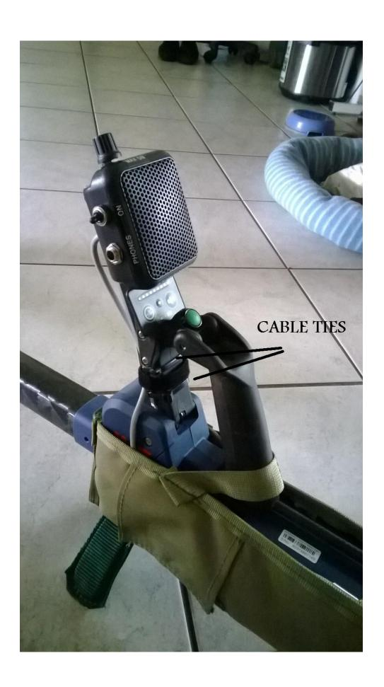
SHOWS HOW TO MOUNT TREASURE MATE BUT USING THE OLDER MODEL OF TREASURE MATE. NEW MODEL HAS NO TOGGLE SWITCH.
