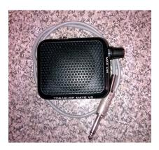
"Treasure Mate Amplifier V.3" to suit VLF / PI Metal Detectors can also be used as utility amplifier for electronic projects.
