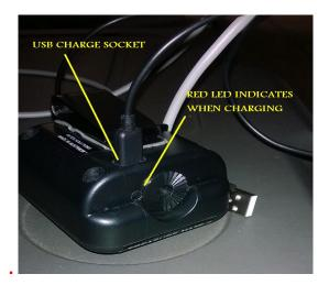
YOU CAN ALSO USE NON-RECHARGEABLE TYPES IN THIS UNIT EG THE ALKALINE 9 VOLT BATTERY.
